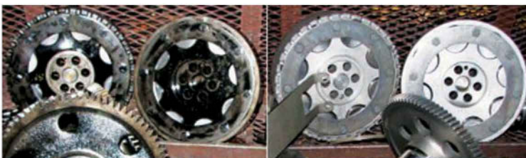
Transmission Parts – before & after cleaning with an aqueous solution
